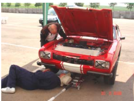
Neil and Mike fixing the Water and Oil leaks discovered in testing.
