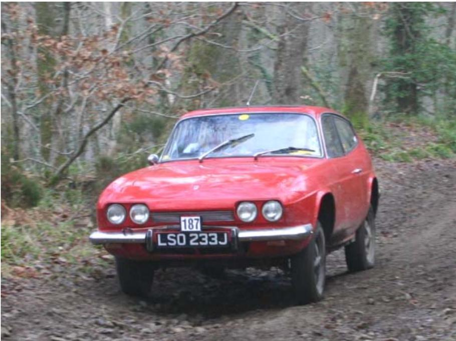
*Dave Nash and Julie Fleet on Fingle in Dave's latest car. It's a Beetle floor-pan with a Torsion Bar front-end and double-jointed rear. Power comes from a Type 4 motor and the whole thing is topped off by a Reliant Scimitar body. Dave had some last minute carb problems but these were resolved and the new car gave very little problem during the event.*
